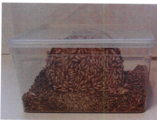
Fig. 3: Exposure of test material FiloSeal+HD Duct Seal (upper left) und MDIII 75n Duct Seal (upper right) against Mastotermes darwiniensis as well as virulence control (lower left).
