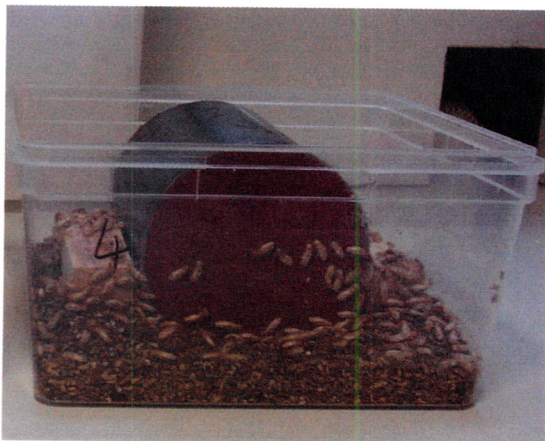
Fig. 2: Top view (left) and frontal view (right) of general test set up before insertion of termites for FiloSeal+HD Duct Seal as example
